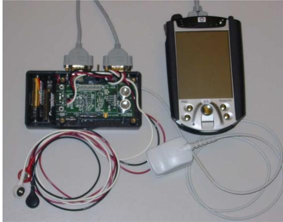
Figure 7.3: Inside the patient waist pack: SpO<sub>2</sub> and ECG sensors, sensor box and HP iPAQ ®.
