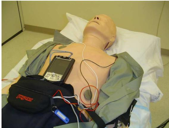
Figure 3.2: Patient simulator wearing PDA and ECG electrodes.
